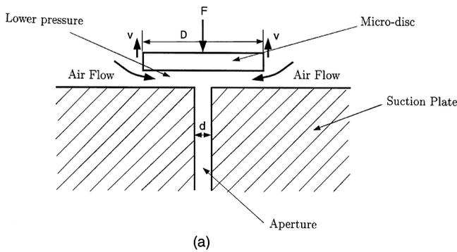
1. Almost two-third of suction force of micro-components is due to lower pressure between the micro-component and the suction plate, because of air viscosity.
