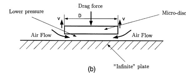
Fig. 5. Schematic representation of (a) lower pressure between the micro-disc and the suction plate, and (b) drag force.
