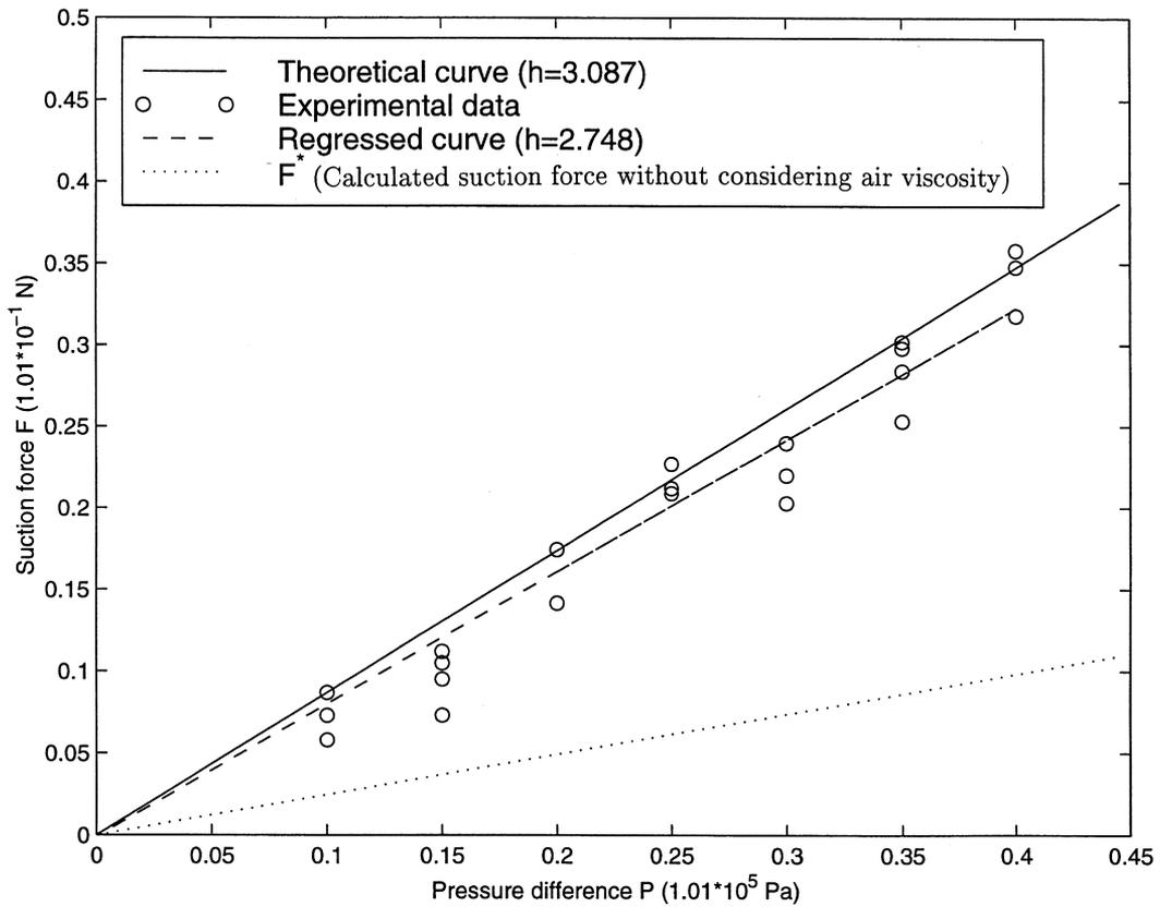
Fig. 4. comparison between theoretical and experimental results of suction force at different values of  $P$ .
