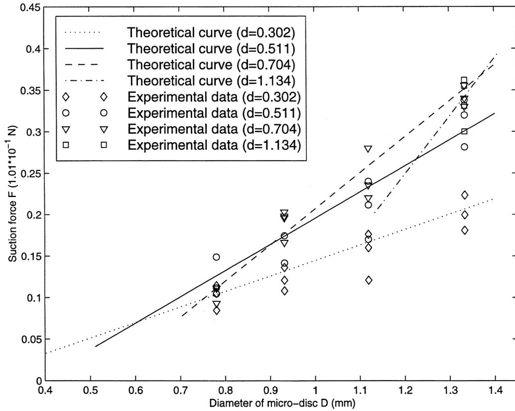
Fig. 2. Comparison between theoretical and experimental results of suction force at different values of  $D$ .
