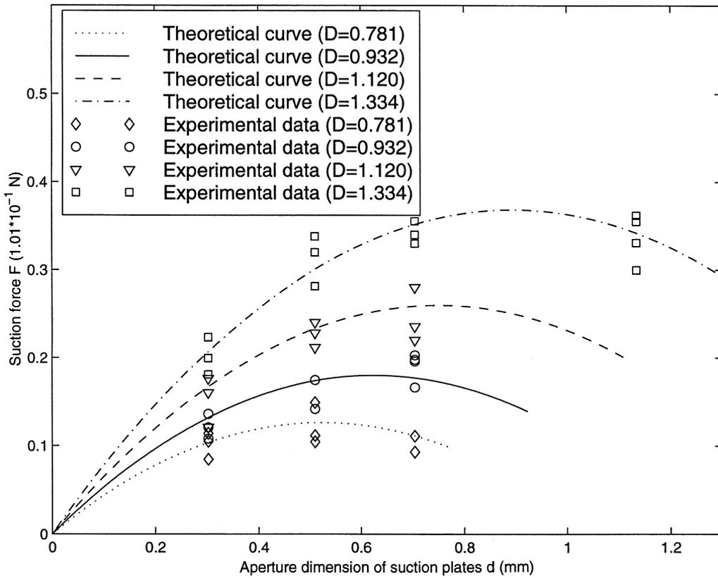
Fig. 3. Comparison between theoretical and experimental results of suction force at different values of  $d$ .
