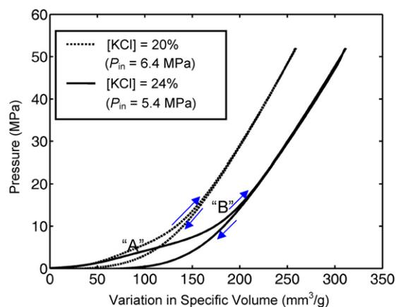
Figure 2. Typical sorption curves at 20 °C.
