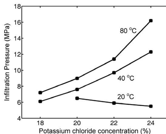
**Figure 4.** The infiltration pressure as a function of the potassium chloride concentration. The data point for 18% solution at 20 °C is not shown since no infiltration can be measured under this condition.
