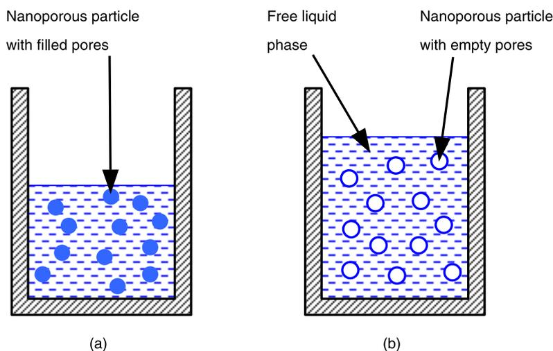
**Figure 1.** Schematic diagrams of the volume-memory liquid: (a) filled nanoporous particles and (b) empty nanoporous particles.
