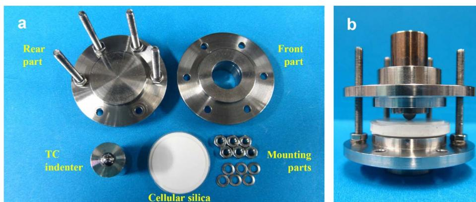
Fig. 2. Indentation testing system. (a) The system components and a cellular silica sample. The diameter of the sample is ~23 mm. (b) A cellular silica sample mounted in the indentation testing system. Part of the mounting parts are removed and the front part is lifted up to show the contact between the indenter and the sample surface.
