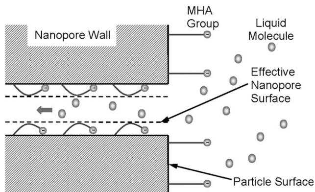
FIG. 2. Schematic of infiltration of liquid phase into a nanopore.
