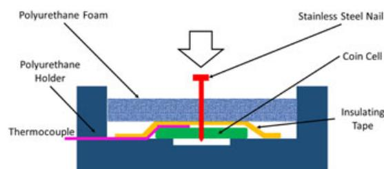
**FIGURE 1** Schematic of the testing system of nail penetration [Colour figure can be viewed at [wileyonlinelibrary.com](http://wileyonlinelibrary.com)]
