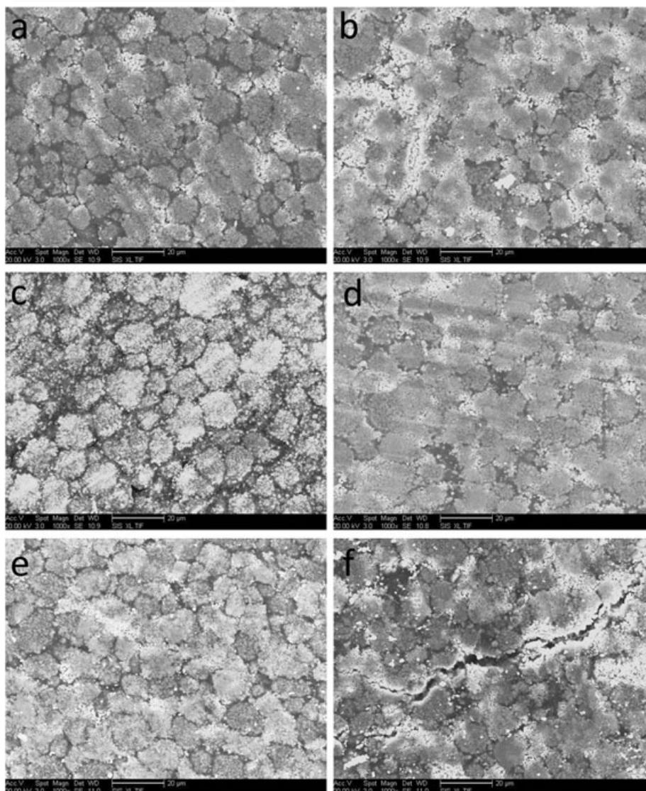
**FIGURE 4** SEM images of reference positive electrodes (A, C, E) and TSB-based positive electrodes (B, D, F) at different stages: after cycling and charging (A,B), after preheating at 110°C (C, D), and after nail penetration, ~0.5 cm away from the nail (E, F)
