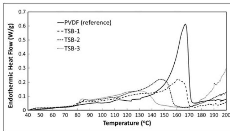
**FIGURE 3** Typical DSC curves of solvent-processed cathode binders
