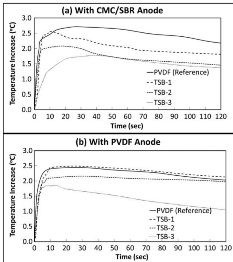
**FIGURE 2** Typical temperature profiles in nail penetration tests of battery cells with anodes bound by (A) 4 wt% CMC/SBR (2:2) and (B) 6 wt% PVDF. The cathode binder is indicated by the legend
