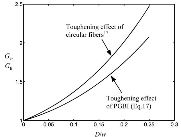
Fig. 4 The relationship between the fracture resistance and the size/spacing ratio of PGBI.
