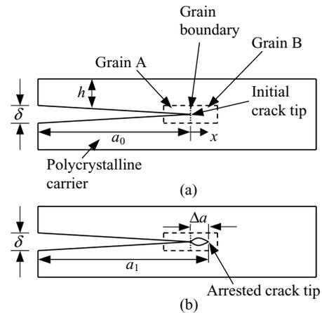
**Fig. 2** A schematic diagram of the double-cantilever-beam specimen (a) prior to the crack jump and (b) after the crack jump.
