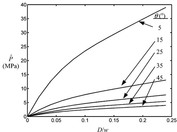
Fig. 5 The bridging force as a function of the  $D/w$  ratio.
