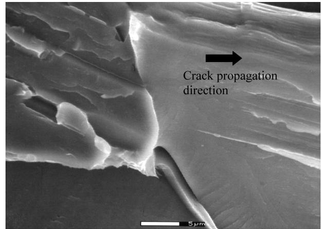
**Fig. 3** SEM microscopy of a PGBI separated through plastic shear at  $-25\text{ }^{\circ}\text{C}$  in an Fe-3wt%Si bicrystal.
