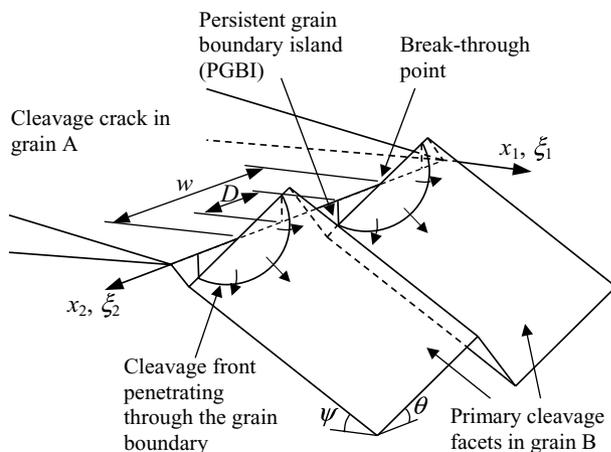
**Fig. 1** A schematic diagram of the cleavage front transmitting across a high-angle grain boundary.
