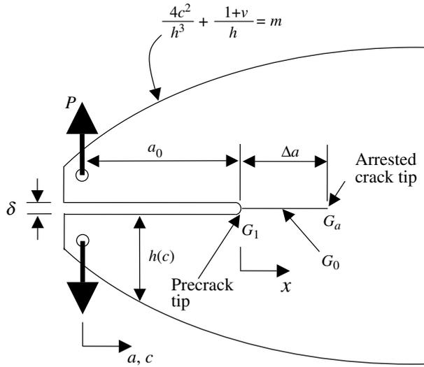
**Fig. 1.** A schematic diagram of the cleavage cracking in a constant- $K$  sample
