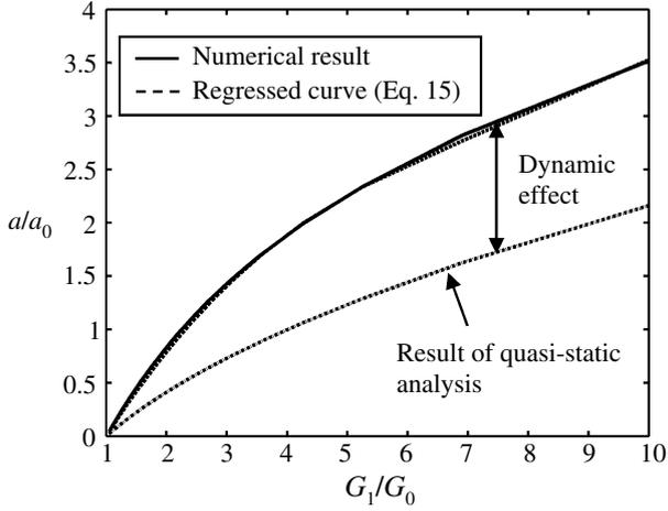
**Fig. 3.** The crack jump length as a function of  $G_1/G_0$
