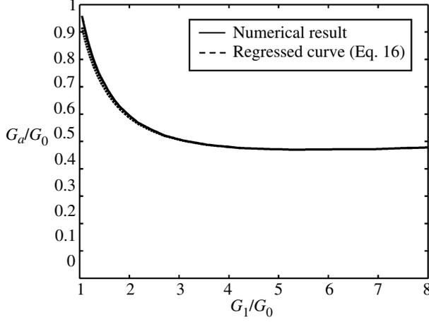
**Fig. 2.** The critical energy release rate of crack arrest,  $G_a$ , as a function of  $G_1/G_0$ , where  $G_a/G_0 = 1/(\tilde{G}\beta)$  and  $G_1/G_0 = 1/\beta$
